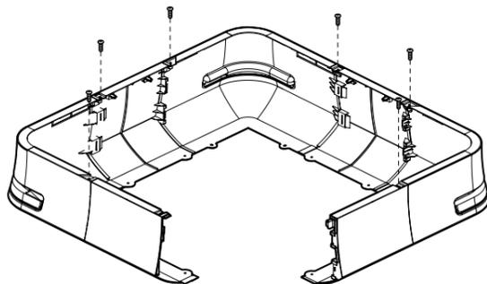
**6** Set the assembled part with cover A and B, and the assembled part with cover C and D to the height of the indoor unit, and tighten the screws. (8 locations)
