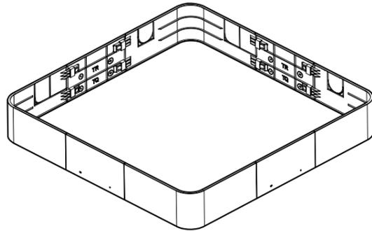
**3** Take one of the 4 covers C and cut out 3 locations for assembly. (Cut out by the groove on the assembly part.)
