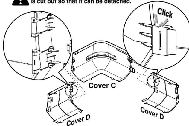
**5** Assemble using cover C and D as shown in the picture and use the provided screws to tighten the covers. (6 locations)
