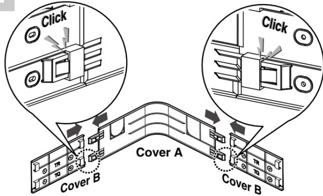
**2** Complete the assembly until the rectangular shape is formed as shown in the picture.
