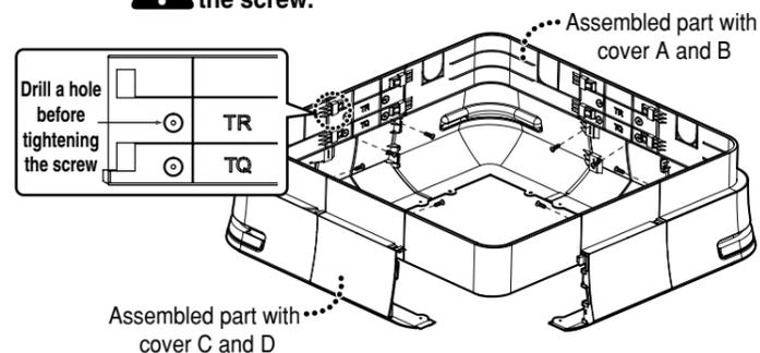
**7** Check the direction of the front panel and set the cover on the panel. (The direction the connecting wire is coming out is the same as the location of the detachable cover.)
