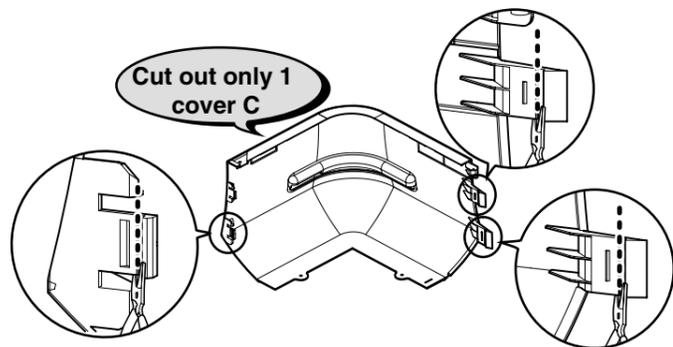
**4** Assemble the remaining 3 covers C and 4 covers D so that they form a rectangular shape as shown in the picture.
