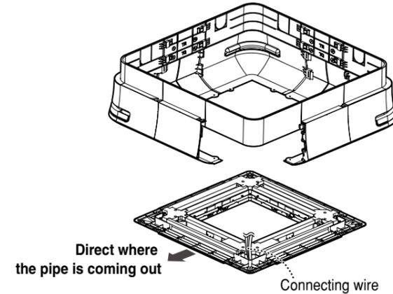
**9** After selecting the direction you want, make holes for pipe and drain hose to fit the installation environment.
