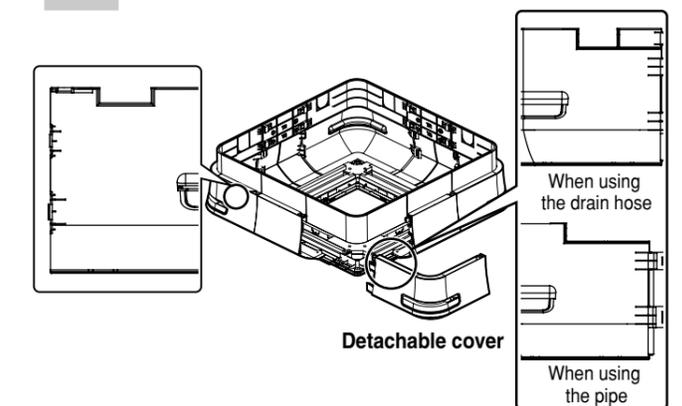
**11** Hold the front panel while keeping it leveled to assemble the indoor unit. (Refer to product installation manual)
